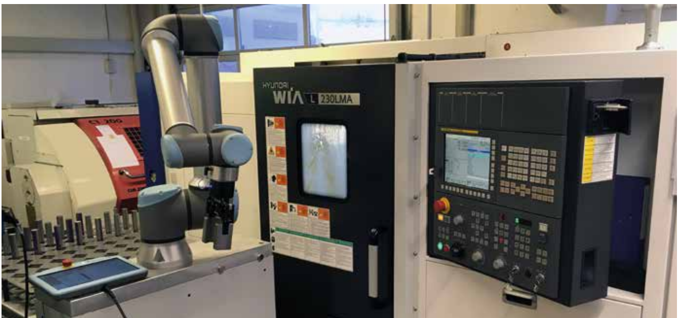
Mobiles Robotersystem SP-MR 1 belädt CNC-Drehmaschine Mobile robot system SP MR 1 loads CNC lathe
