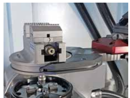
Mechanischer Zentrischspanner MZQ 170-60 PA, Erowa ITS 148 Mechanical centre-clamping vise MZQ 170-60 PA, Erowa ITS 148
