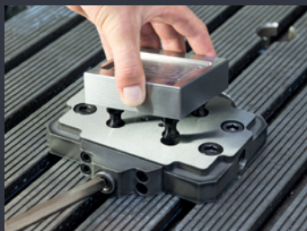
4x ZPS clamping unit mounted on the machine table
